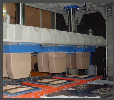
This machine is designed to cast two parts water tank. Each mould is divided two cavities. Bottom part of the mould is fixed on the machine
